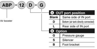
Note) Option G (pressure gauge) is installed onto air booster at shipment. B (foot bracket) and S (silencer) are attached.
