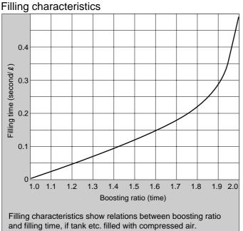
To find filling time, when filling tank with air, where secondary side air pressure
